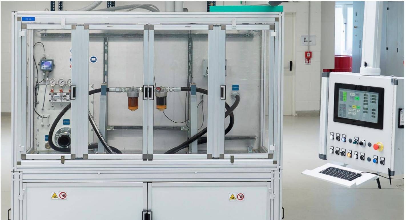
The specific hydraulic system and the instruments used are capable of measuring and recording the electrical potential generated when a filter is crossed by a flow of oil, measured in kV.
