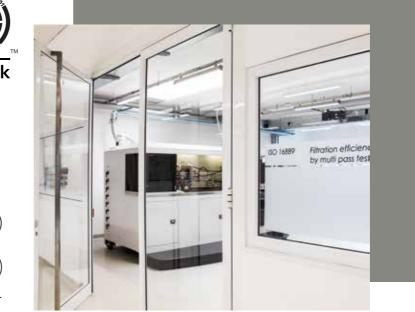
Supported by the latest technology, including scanning electron microscopes, MP Filtri's exhaustive testing program is carried out with special emphasis on its comprehensive MULTIPASS analysis – which has been created in accordance with ISO16889. This method compares the amount of contaminant present upstream and downstream in the filter element – calculating the ratio of Beta filtration by the size of the particles and retention capacity.
