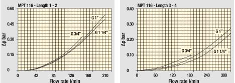
Bypass valve pressure drop
