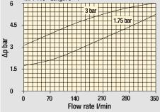
The curves are plotted using mineral oil with density of 0.86 kg/dm<sup>3</sup> in compliance with ISO 3968. Δp varies proportionally with density.
