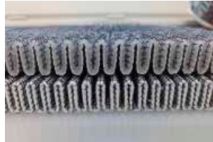
The Filter Media has absorbed water
