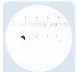
NAS 6 ISO 17/15/12 Typically Required for most modern hydraulic systems
