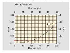
Filter housings ∆p pressure drop. The curves are plotted using mineral oil with density of 0.86 kg/dm³ in compliance with ISO 3968. ∆p varies proportionally with density.
