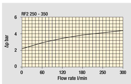
Bypass valve pressure drop
