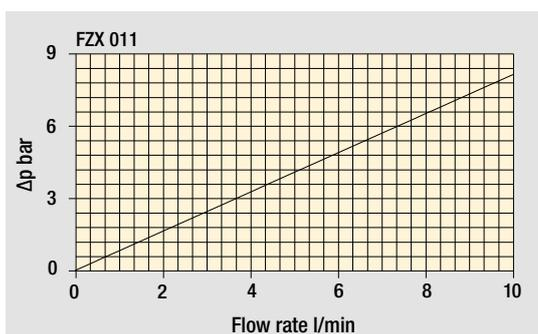
The curves are plotted using mineral oil with density of 0.86 kg/dm<sup>3</sup> in compliance with ISO 3968.  $\Delta p$  varies proportionally with density.
