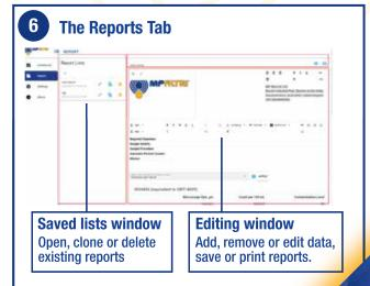
Enables operators to create reports for both historic and current data. Results can be saved in different formats such as pdf, or printed hard copy. Reports which are no longer needed can be cleared, or even deleted from this Tab.
