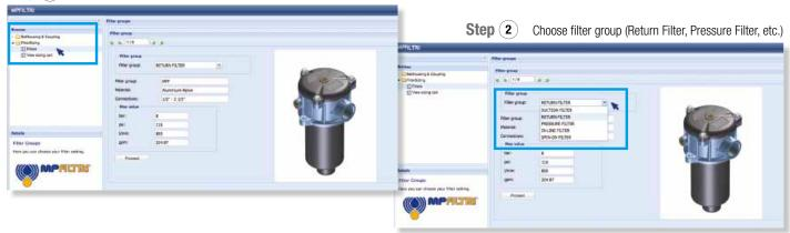
Choose filter type (MPF, MPT, etc.) in function of Step (3) the max working pressure and the max flow rate
