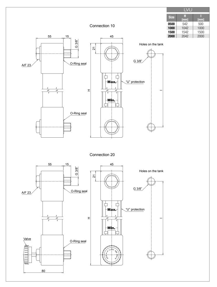
Electromagnetic float level indicators use the action of a magnet fixed to the float to change the electrical status of a reed switch mounted inside the tube.
