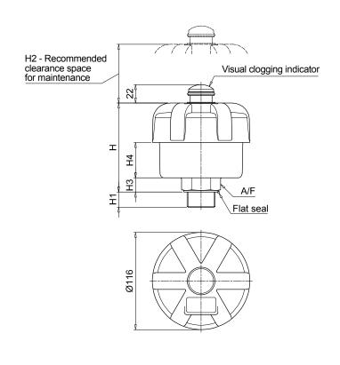
The filler plugs series is composed by different versions: with breather filter, with dipstick for measuring the reservoir fluid level or with anti-splash fins to prevent spillage of oil from the reservoir to be specifically used on mobile equipments.
